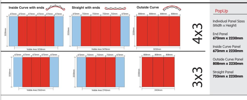
A stand is described by the number of frame squares wide (panels) x the number of frame squares high. Standard panel height of 2230mm increases to 2963mm for a 4-squares high frame, 3696mm for 5-squares high, and 4429mm for 6-squares high. Additional stabilising is recommended for increased heights, using either weights or our unique Frame Support Brace.
